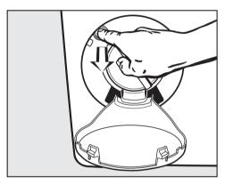
■ Pull the emergency release (see illustration). The loading door will open.
